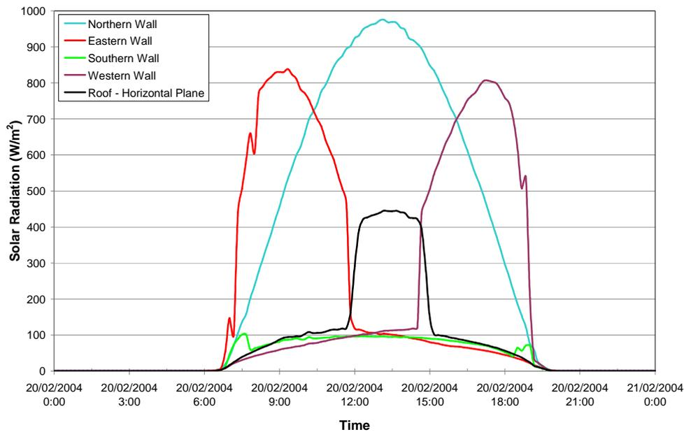
**Fig. 1. The solar irradiance for external surfaces of modules on a summer day [1]**
