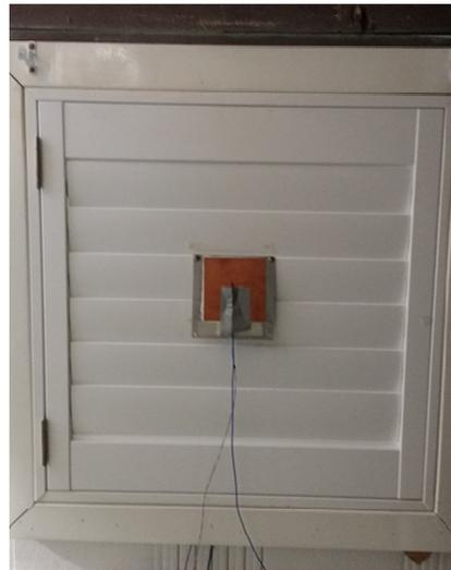
**Fig. 4. Heat flux sensor fixed on back of a panel**
